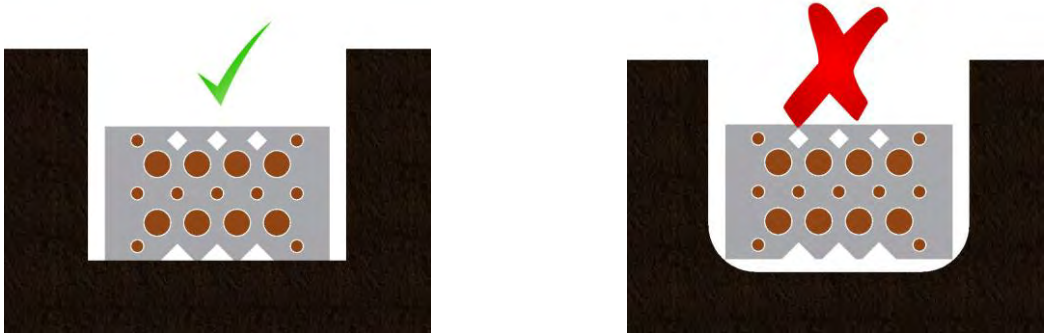
End View of Conduit Trench
